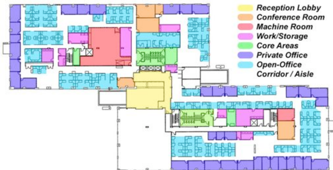
Figure 1. Floor Plan: Office Building Typical Floor Showing Types and Distribution of Spaces.
